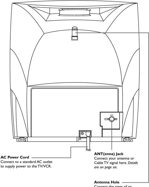
Connect the stem of an indoor rod antenna here. Details are on page six.
